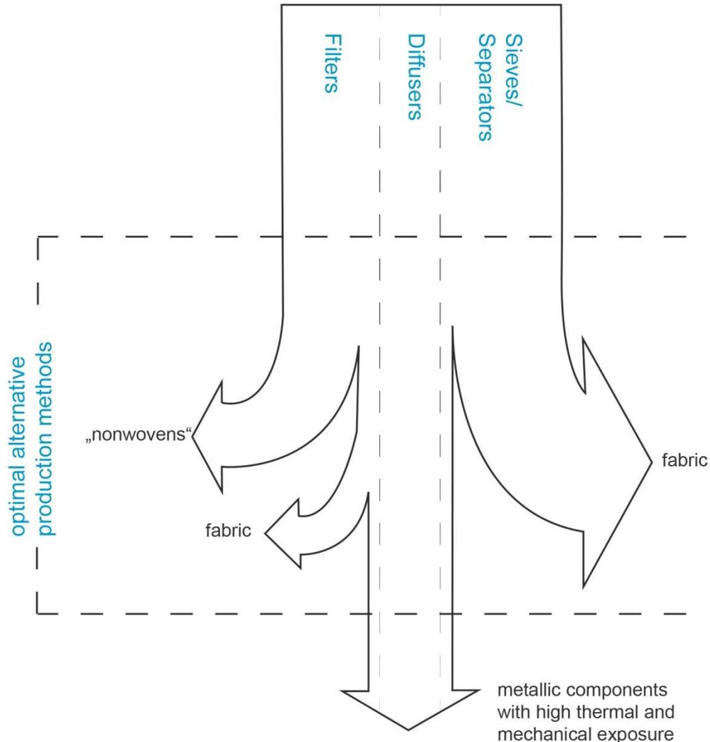
Fig.1: Production technique for filters, sieves and diffusers
