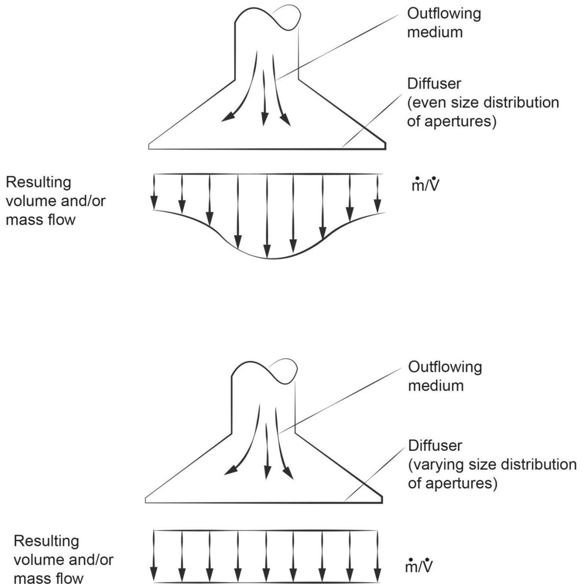
Fig. 6: Compensation of flow effects by varying the aperture shape or size
