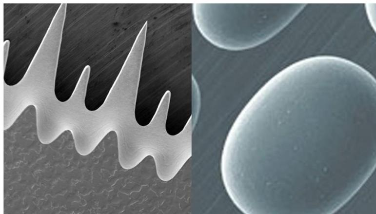
Fig. 4: Geometries produced by photo chemical etching at consistent productivity
