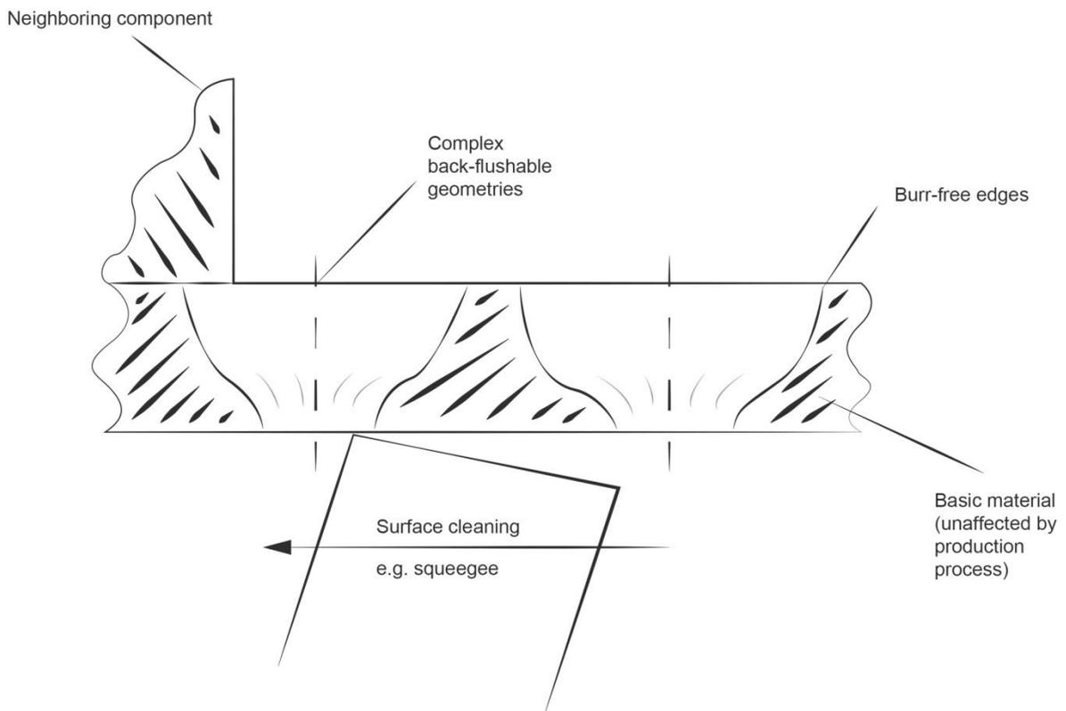
Fig. 3: General advantages of chemical etching
