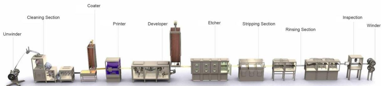
Fig. 2: Industrial metal etching - continuous chemical etching technology
