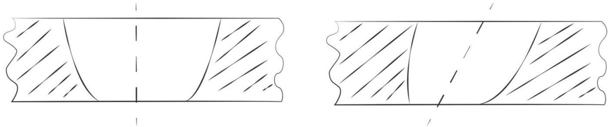
Fig. 5: Variants of back-flushable shapes
